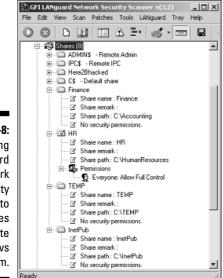
Figure 7-8: Using LANguard Network Security Scanner to find shares on a remote Windows system.
