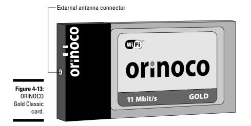
The ORiNOCO Gold Classic card from either Agere or Lucent is a popular card with wireless hackers because it has an external antenna connector and works with both Kismet and NetStumbler. Take care when buying new ORiNOCO cards. ORiNOCO is now owned by Proxim, which came out with an ORiNOCO card *not* based on the Hermes chipset. The Hermes card is still available, but it is usually sold as the ORiNOCO Gold Classic.
