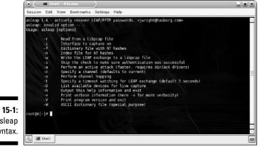
Figure 15-1: The asleap syntax.
